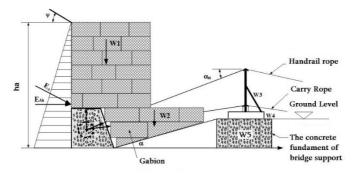
Fig. 3. The device of the "gravitational" anchor of the bearing cable of the suspension bridge using gabions.
