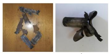
a b Fig. 4 Typical images of steel tube fragmentation (a) and deformation (b) after explosion a - I substance b - II substance
